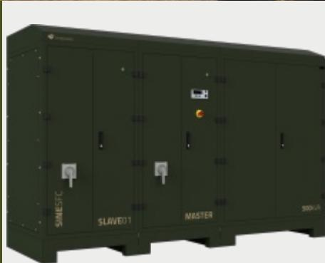
SINEPOWER manufacture a variety of Static Frequency Converters. Static Frequency Converters convert the source power with a specific input voltage and frequency in to a different output voltage and frequency depending on what the client requires.
